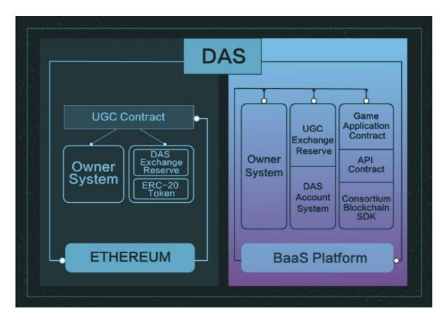
ugChain Digital Asset Management System (DAS) based on double-chain technology and consists of four contract subsystems, UGC Contract, DAS Account Contract, DAS API Contract and BaaS Platform, which can provide secure and stable operation support for ugChain digital asset management applications and game applications.
